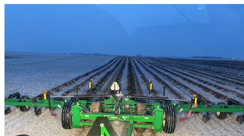
Figure 4. Field operation and field finish of a Deep Ripping application. .
